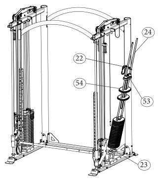
**STEP 4 A.** Insert the **Guide Rods (24)** through the holes in the bottom of the frame. Be sure the ends of the rods with the holes are facing **Up**.
