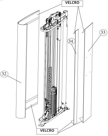
STEP 7 D With all Shrouds in place, tension covers by turning **bolts (15)(38)(39)** at top of the frame.
